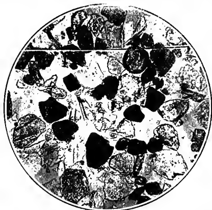
FIG. 17. Fine sand, photomicrograph. Magnified about 110 diameters. Differences in color indicate differences in mineral composition. Each particle composed of one mineral.
